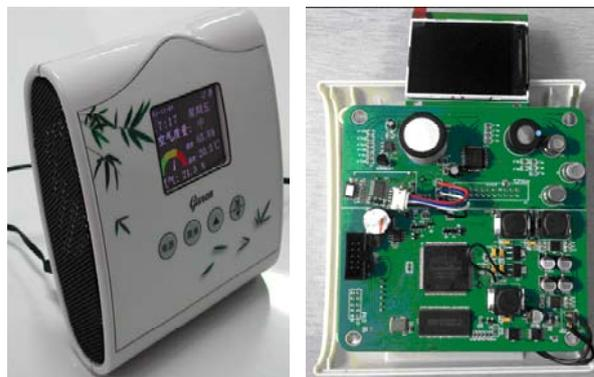
Fig. 1. Photograph of the implemented E-nose (left), and inside components (right),
