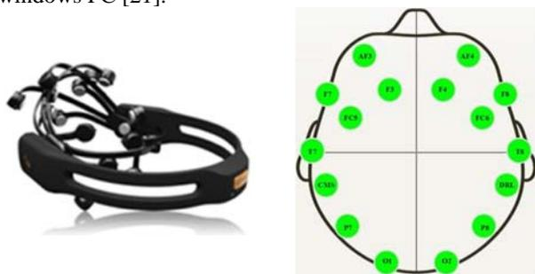
Fig. 2 Signal acquisition unit: the Emotiv EPOC headset (Left) and the location of electrodes relative to the head (Right).
