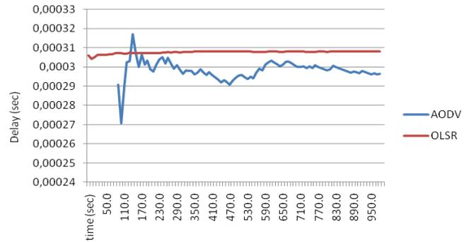
Fig. 4 End-to-end delay 30 nodes AODV vs. OLSR (with attack)
