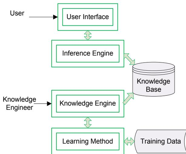
Fig. 1 Architecture of the inductive expert system.
