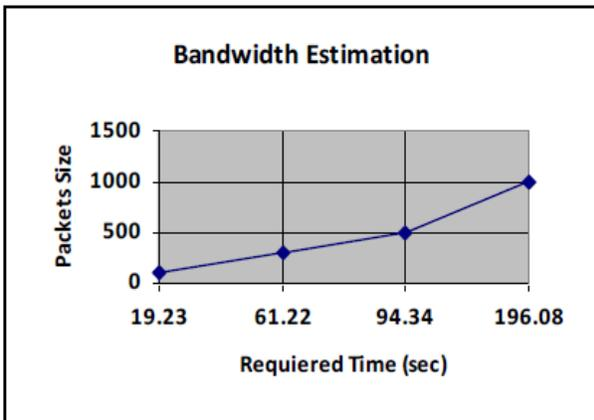
Figure2: LAN 10Mbps bandwidth measurement (Afternoon)
