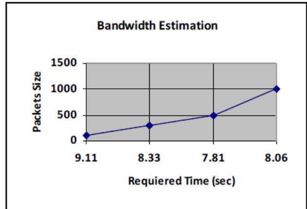
Figure3: LAN 10Mbps bandwidth measurement (Midnight)
