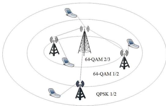
Fig.4 The typical topology of relay network [9, 10]
