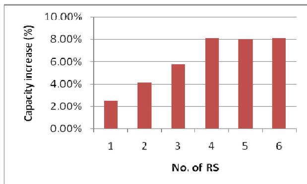
Fig. 12 Capacity increase vs. number of RS
