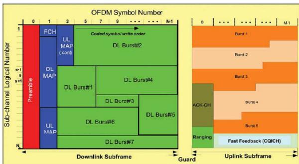
Fig. 1 WiMAX OFDMA TDD Frame Structure [1].
