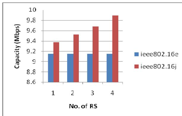
Fig. 11 Capacity vs. number of RS
