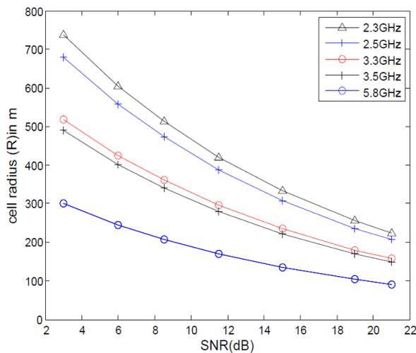
Fig. 9 Cell radius vs SNR
