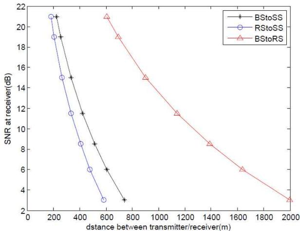
Fig. 6 Distance vs. SNR
