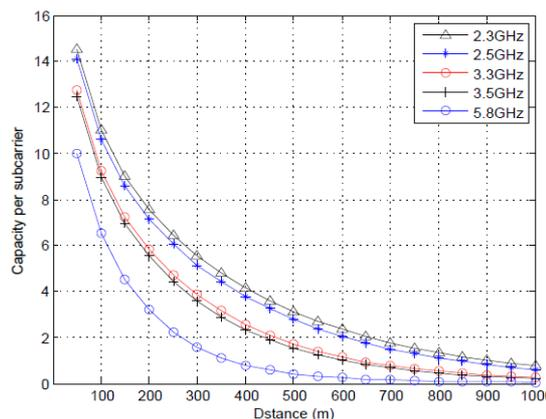
Fig. 10 Capacity per subcarrier vs distance
