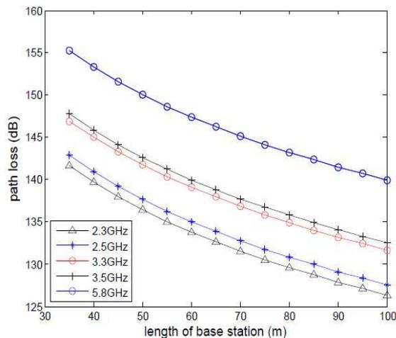
Fig. 8 Path loss vs length of base station
