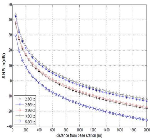
Fig. 7 SNR vs distance
