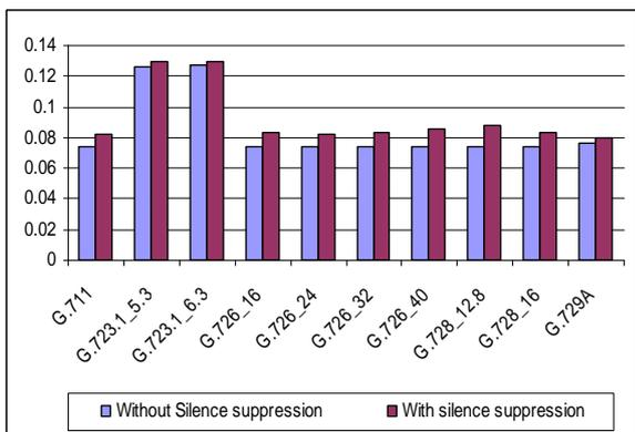
Fig.6 Packet End to End Delay with silence suppression (sec)
