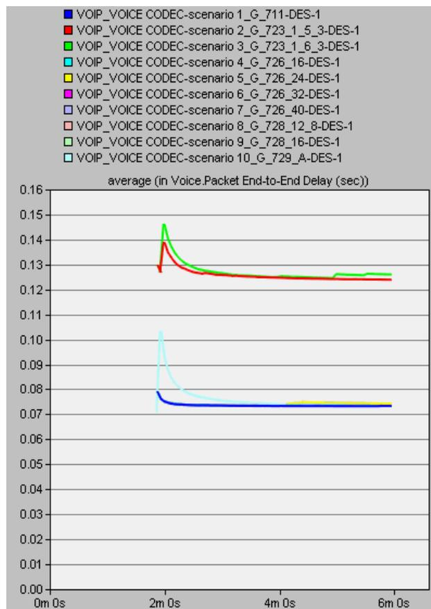
Fig.2 Relative Packet End to End Delay of voice codecs (sec)
