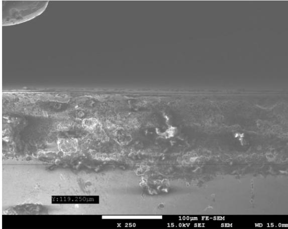
Fig. 5: The boundary between work-hardened and non-hardened material
