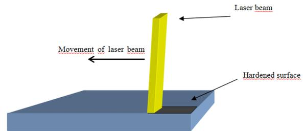
Fig. 2: Robot laser hardening with different temperature and speed
