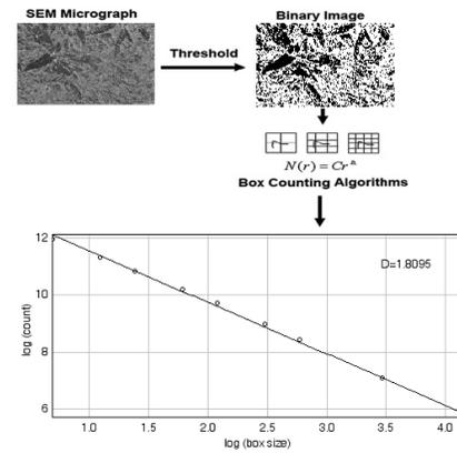
Fig. 6: Calculation of fractal dimensions with box-counting method
