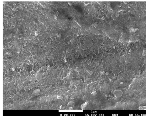
Fig. 4: SEM picture of robot laser re-hardened specimen
