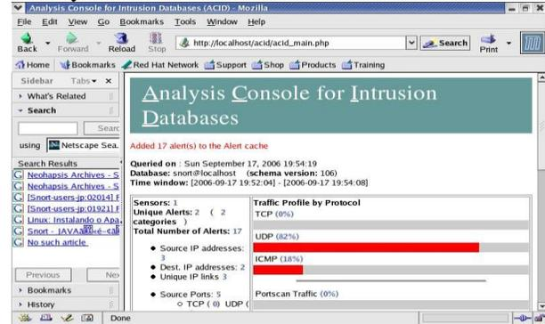
Fig. 7 Snort output using Acid
