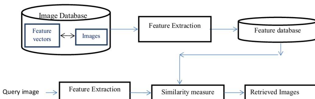
Fig (1) An architecture of a content-based image retrieval system.
