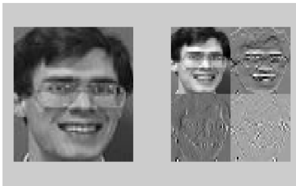
Figure 3: The decomposed image in 1 level DWT
