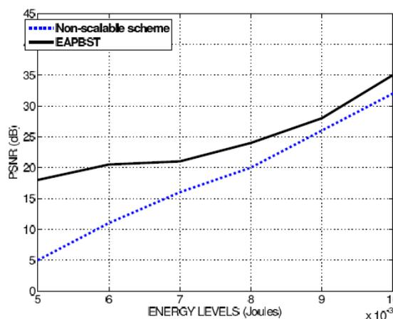
Fig. 4. Graph showing the distortion response in relation to energy budgets
