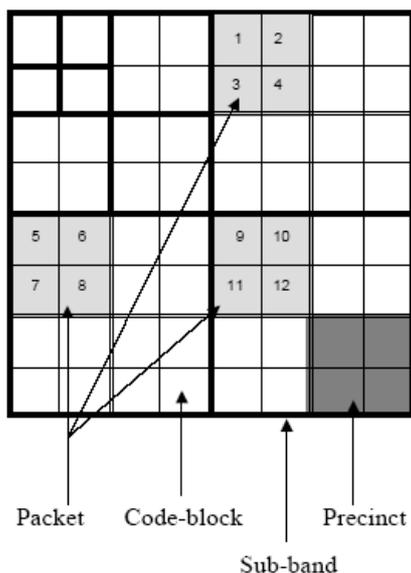
Fig 2: JPEG 2000 code blocks and partitions in JPEG 2000.
