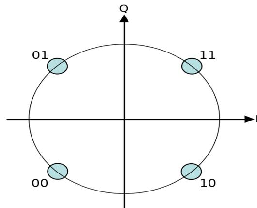
**Fig. 1.2: Signal Constellation Diagram for 4-PSK**
