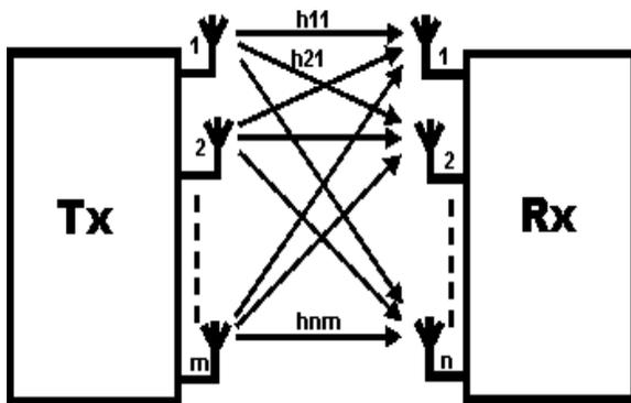
**Fig. 1.1: Basic representation of M X N MIMO System**
