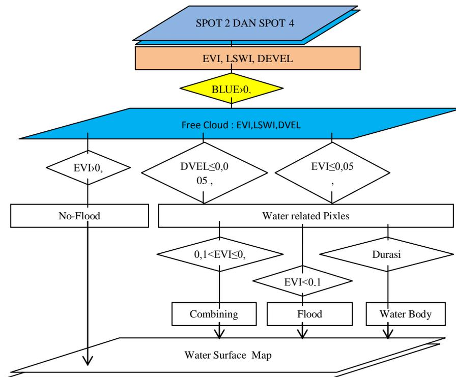
Figure 2 Flowchart of Optical Image Segmentation by EVI and LSWI
