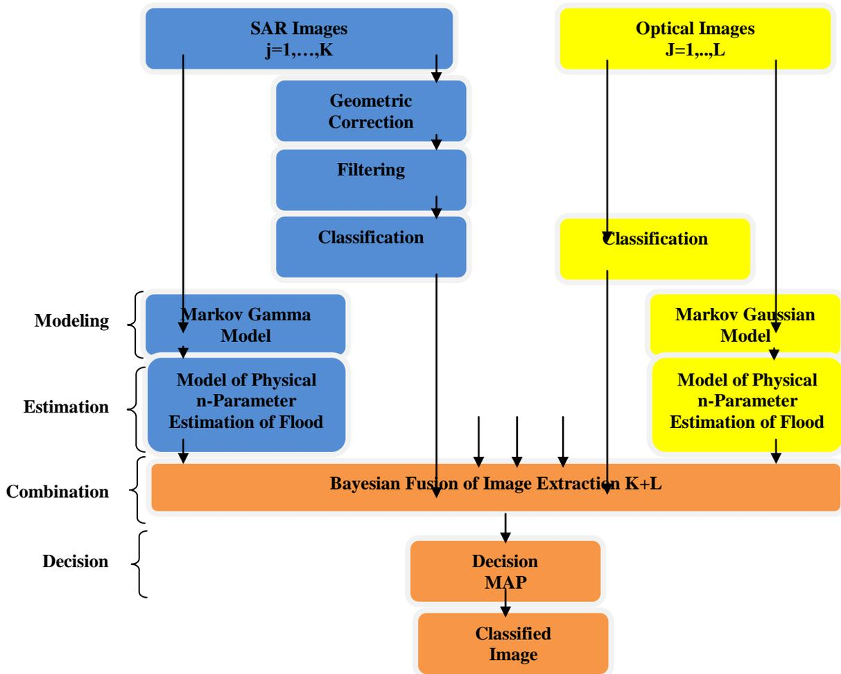
Figure 1 The Approach of Probabilistik Multisource Fusion for Flood Detection
