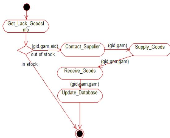
Fig. 2. an activity diagram of ordering system
