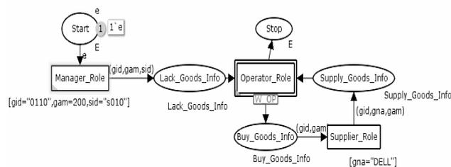
Fig. 4. the prime HCPN model of ordering system
