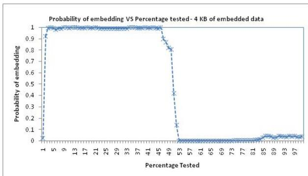
Fig. 5 Chi-square result of Simple LSB method for embedding 4KB data.
