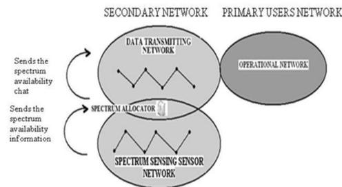
Fig.2 Proposed network architecture of cognitive sensor system.
