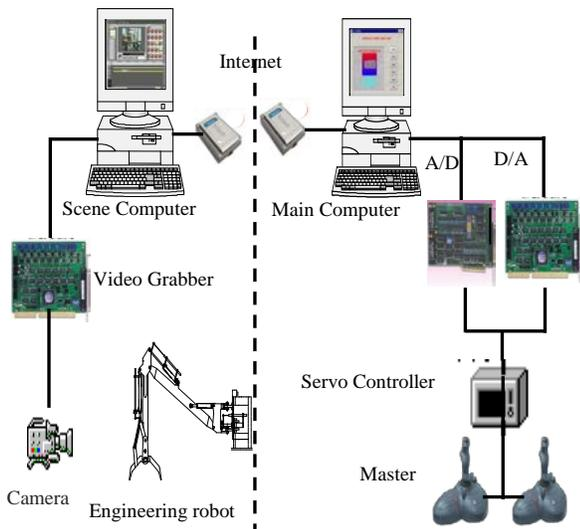
Fig. 2 Master-slave system for remote control
