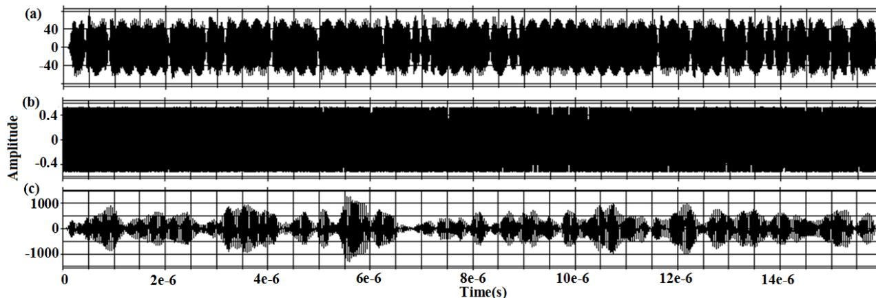
Fig. 7 The export wave: (a) of transmitter; (b) after once frequency conversion; and (c) after twice frequency conversion. Note that (a), (b) and (c) have the same horizontal axis.
