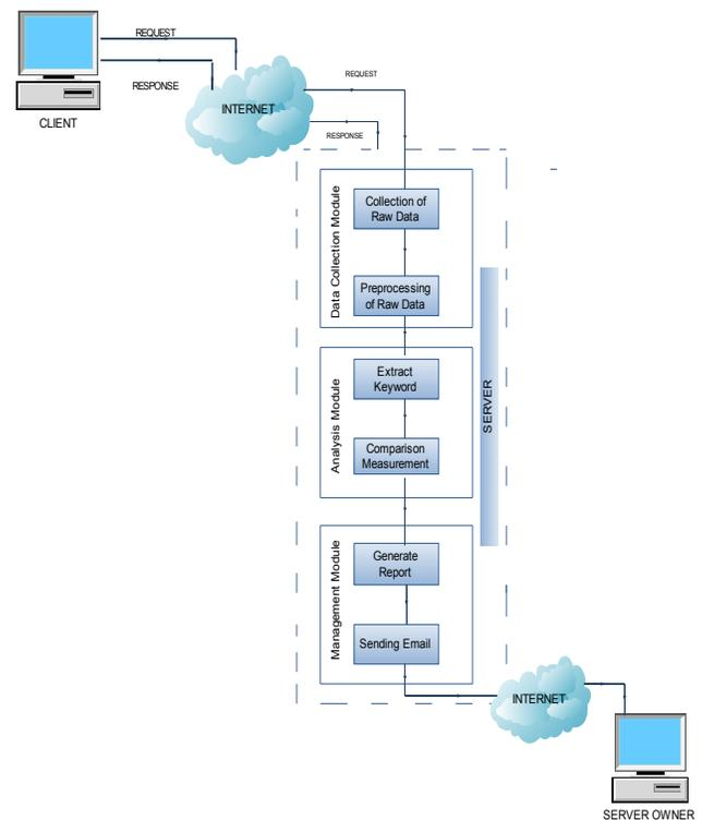
Fig. 1 Block Diagram of Proposed Enhanced IDS
