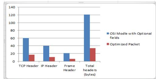
Fig. 9 comparison chart between OSI headers (TCP) with optional fields and optimized packet headers
