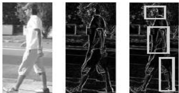
Fig 3: Left: an image window. Middle: the edge magnitude.
