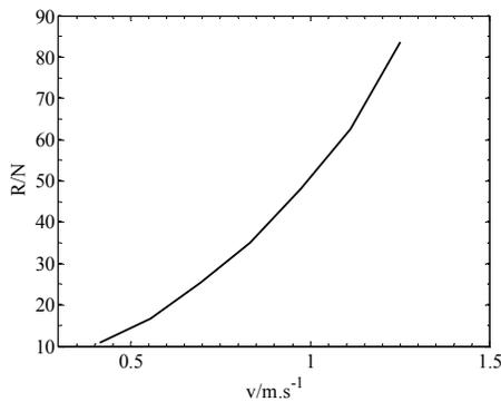
Fig. 1 Model test of the resistance curve
