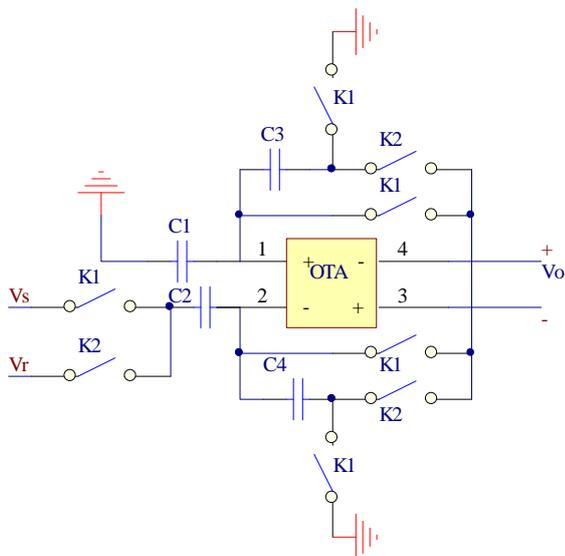
Fig 4 The interface circuit between CDA and PGA
