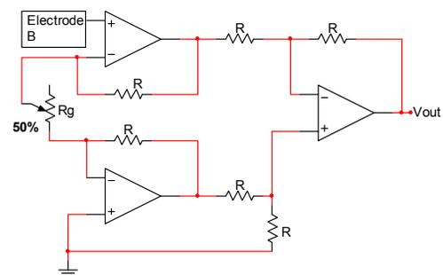
Fig 7. Instrumentation amplifier
