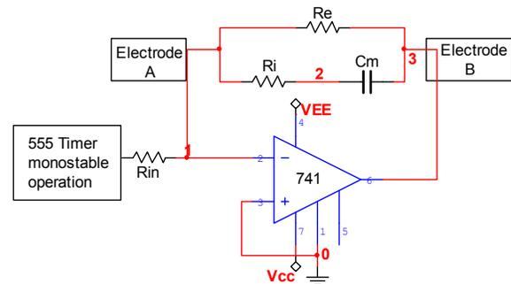
Fig 6. Current pulse generation
