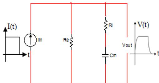
Fig 3. EIS by current injection and voltage detection
