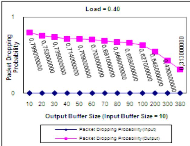
Fig. 4.1 Packet dropping probability in input and output buffers for load=0.4 (M/M/1/K)
