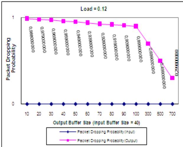
Fig. 4.6 Packet dropping probability in input and output buffers for load=0.12 (Self-Similar)
