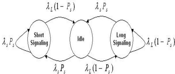
Fig. 3.2 Three-State Signaling Arrival Process
