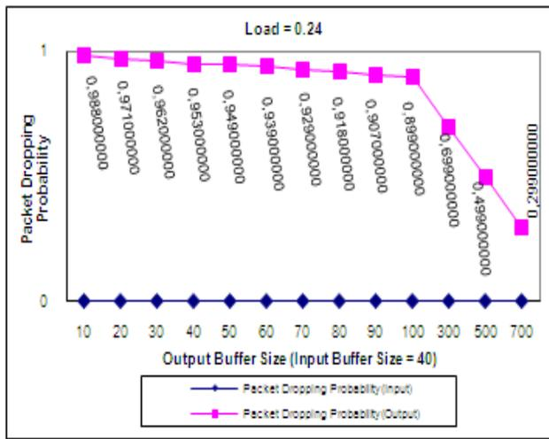
Fig. 4.5 Packet dropping probability in input and output buffers for load=0.24 (Self-Similar)
