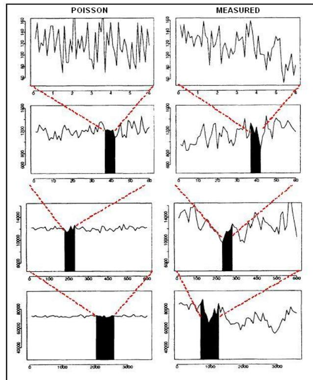
Fig. 3.1 Comparison of the self-similar Internet traffic (measured) with Poisson [8]
