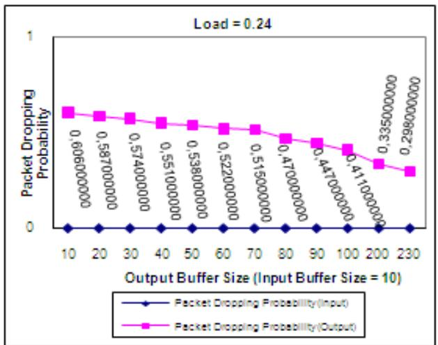
Fig. 4.2 Packet dropping probability in input and output buffers for load=0.24 (M/M/1/K)
