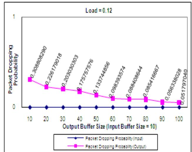
Fig. 4.9 Packet dropping probability in input and output buffers for load=0.12(MMPP/C2/1/K)
