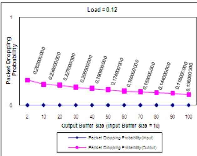
Fig. 4.3 Packet dropping probability in input and output buffers for load=0.12 (M/M/1/K)
