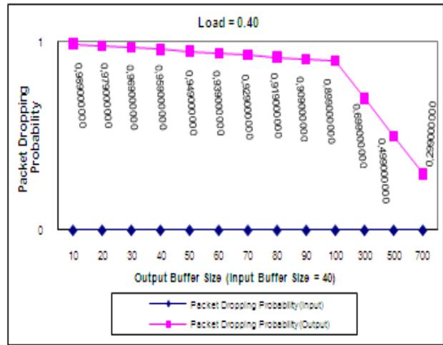
Fig. 4.4 Packet dropping probability in input and output buffers for load=0.4 (Self-Similar)
