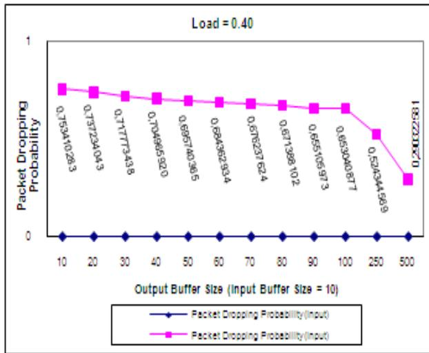
Fig. 4.7 Packet dropping probability in input and output buffers for load=0.4(MMPP/C2/1/K)
