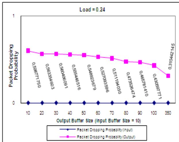
Fig. 4.8 Packet dropping probability in input and output buffers for load=0.24(MMPP/C2/1/K)
