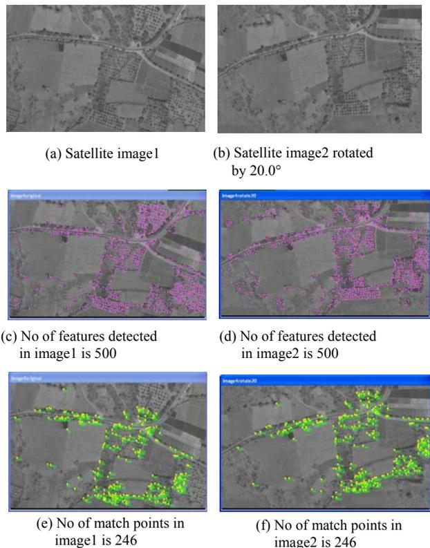
Fig. 8 (a – f) Feature extraction, reduction, matching for a pair of satellite images
