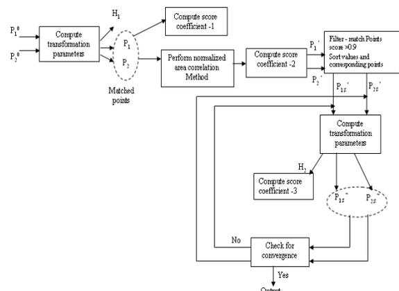
Fig.1 Block diagram for iterative registration procedure
