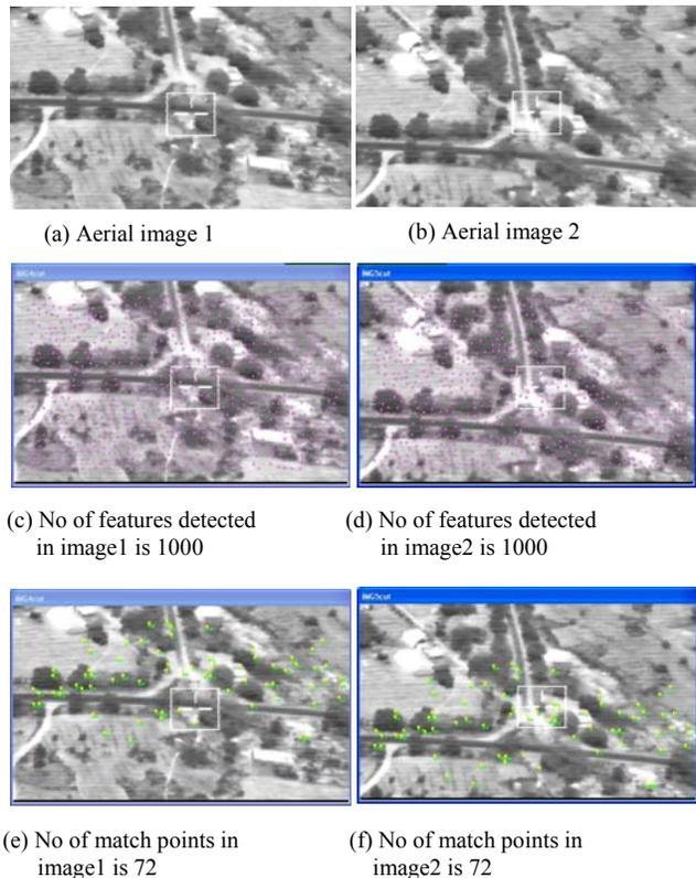
Fig. 10(a)-(f) Feature extraction, reduction, coarse & fine matching for a pair of aerial image-Road Junction
