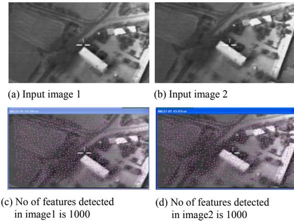
Fig. 2(a) – (d) Input images and feature detected images using KLT corner detector
